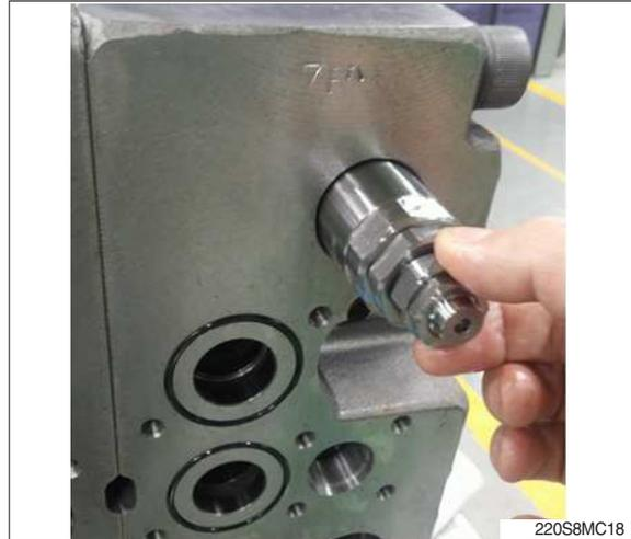
**(10) Disassembling of port relief valve (Except the option side)**
