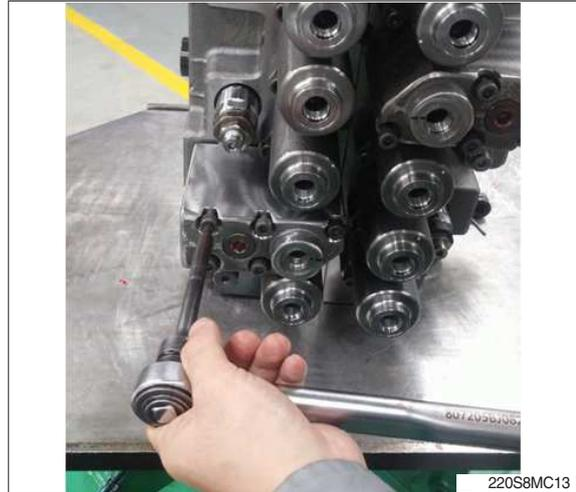
**(5) Disassembling of bypass cut spool (=BC)
