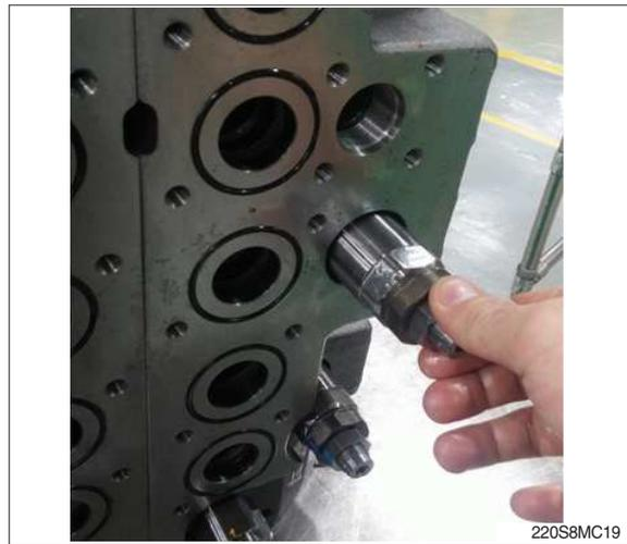
**(11) Disassembling of port relief valve (Option side)
