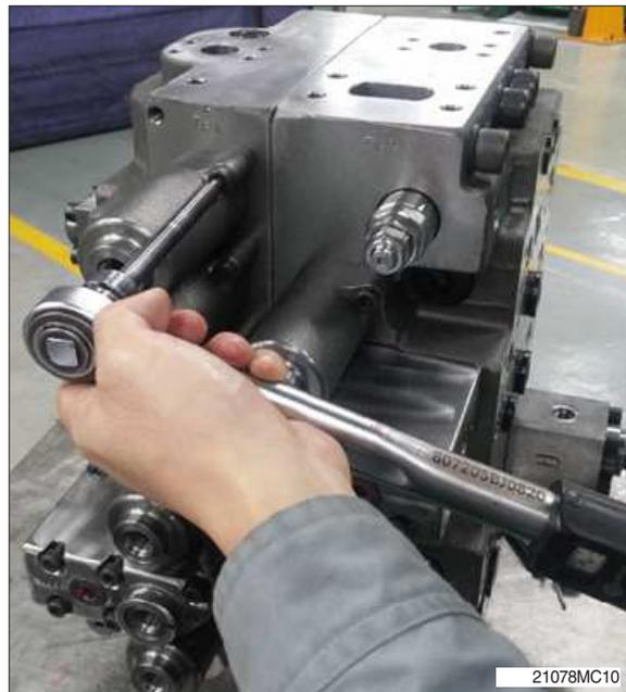
**(4) Disassembling of main spool assy 2 (Pilot cover B side)
