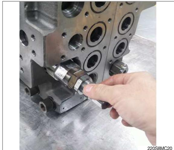
(12) Disassembling of logic valve
