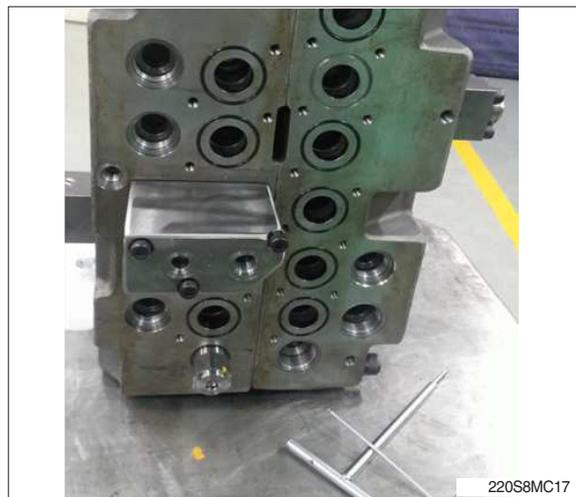
**(9) Disassembling of main relief valve**
