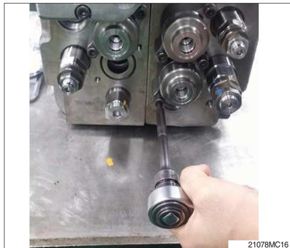
**(8) Disassembling of regen valve block assy**
