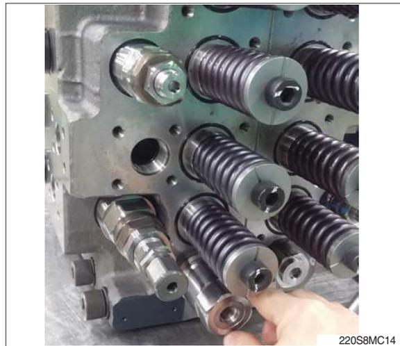
**(6) Disassembling of pilot cover (Bucket stroke limiter)**
